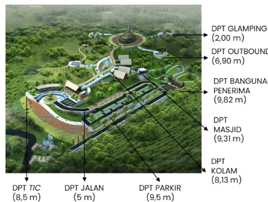
Figure 23. Land Filling and DPT Placement Concept
